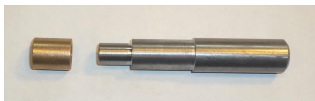
New 'Oilite' bush and bespoke drift
