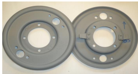
Backplates cleaned and etch primed
