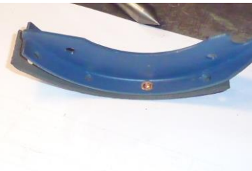
Rivet closed with drift
