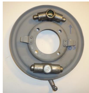
Actuator & adjuster in position
